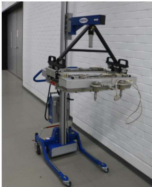
Figure 16:AT93000 twinning lift described in the Advantest documentation
